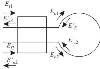
Note that  $kl = \pi/4$  for a 3-dB coupler. Using this and ignoring the common phase factor  $e^{-i\beta l}$ , we get
