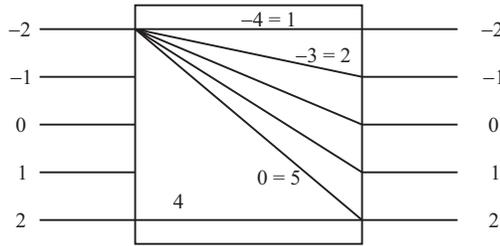
By renumbering the wavelengths, the static router can be assumed to use wavelength  $\lambda_{(i+j) \bmod N}$  to connect input  $i$  to output  $j$ . The figure above shows the renumbering for  $N = 5$ . Thus if  $(i+j) < 0$ , the wavelength used is  $\lambda_{i+j+N}$ . For example, input  $-2$  uses wavelength  $-2 - 2 + 5 = 1$  to connect to output  $-2$ . Thus  $\Delta\theta$  must satisfy
