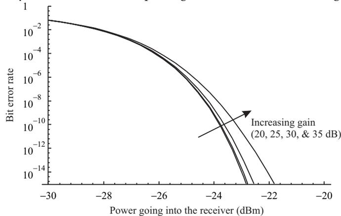
Here we plot the BER versus the signal power going into the receiver for  $P = -30$  dBm for  $G = 20, 25, 30,$  and  $35$  dB. For  $G$  in the 20–30 dB range, the curves are very close to each other. For  $G = 35$  dB, the signal-spontaneous noise begins to dominate and the BER increases for the same signal power into the receiver.
