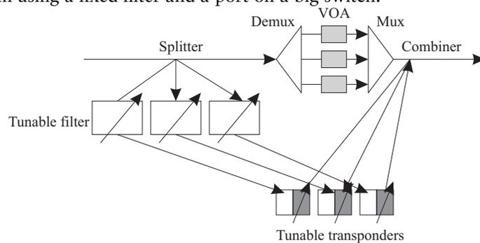
Another plausible OADM architecture is shown above. Here a wavelength blocker device (a demux/mux combination with a per-channel variable optical attenuator) is used to either block the add/drop channels from passing through as well as equalize power levels for the passthrough channels. The loss in the passthrough path is low, but the loss in the add/drop path is high due to the splitters and combiners. However, tunable filters need be provided only for drop channels and not for all channels.
