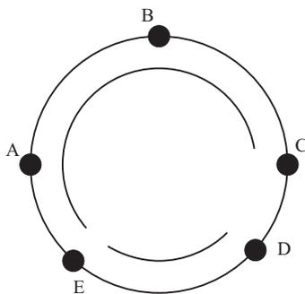
Next consider a 1 hop connection DE. If link DE fails, both path and line protection use DCBAE to restore the connection. In this case, both need the same amount of bandwidth for restoration. In general, path protection is better (more efficient use of bandwidth) at restoring multihop connections than line protection.
