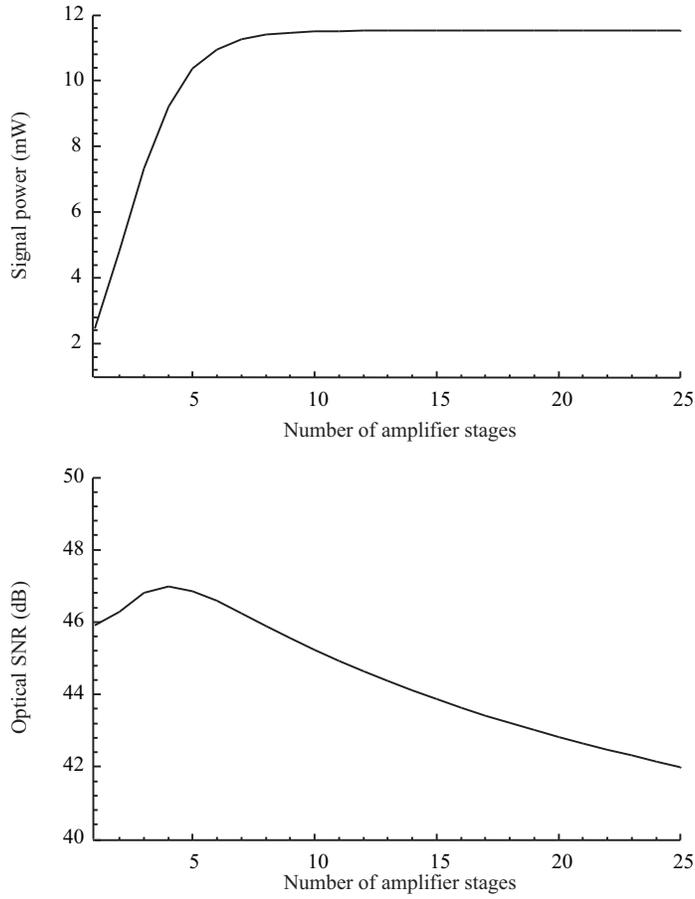
Note that the signal power reaches its steady state value of 11.5 mW calculated above, after a few stages. The optical SNR increases for the first few stages but later decreases with increasing number of stages, due to accumulation of noise at each stage.
